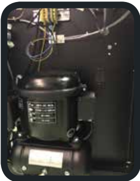
Silent compressor inside the machine
