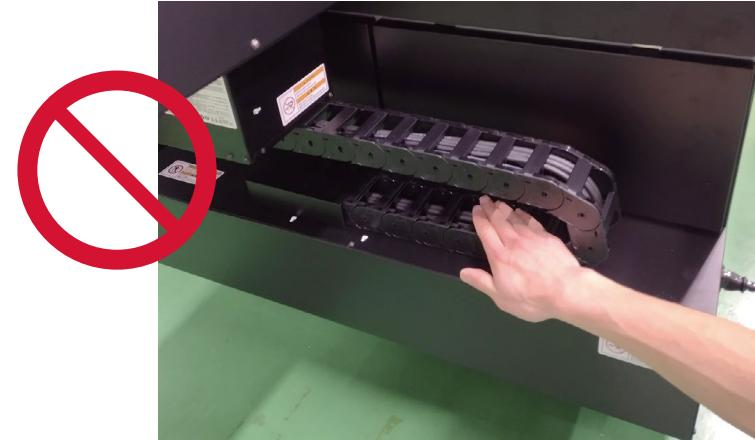
Keep away from the area that the gantry moves while printer is in operation.
