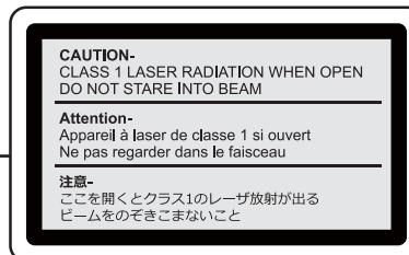
Laser Cautions Label for Access Panel
