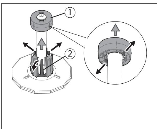
(If you are using 2-inch core roll media) Remove the 3-inch adapters from the media flange.
