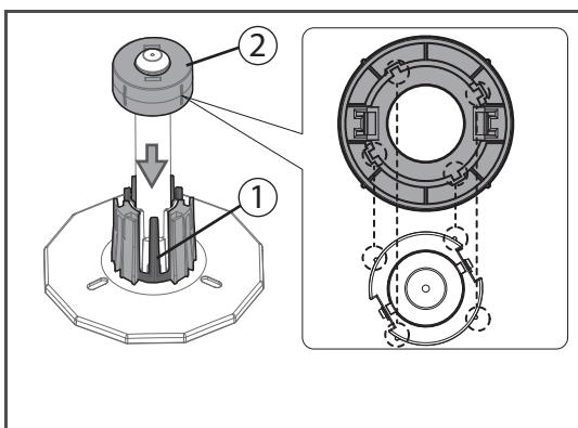
(When replacing 2-inch core roll media with 3-inch core roll media) Attach the 3-inch adapters to the media flange.
