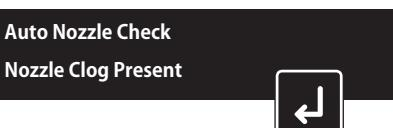
If the printer is unable to select a print head or a nozzle segment that works properly even after 3 cleanings, the message "Auto Nozzle Check Nozzle Clog Present" will appear on the operation panel.
