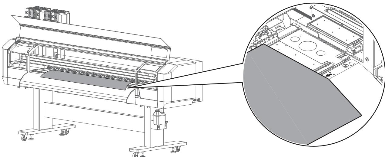
[8] If needed, use a slide lock lever on the pressure rollers to individually cancel or reduce the holdown pressure.
