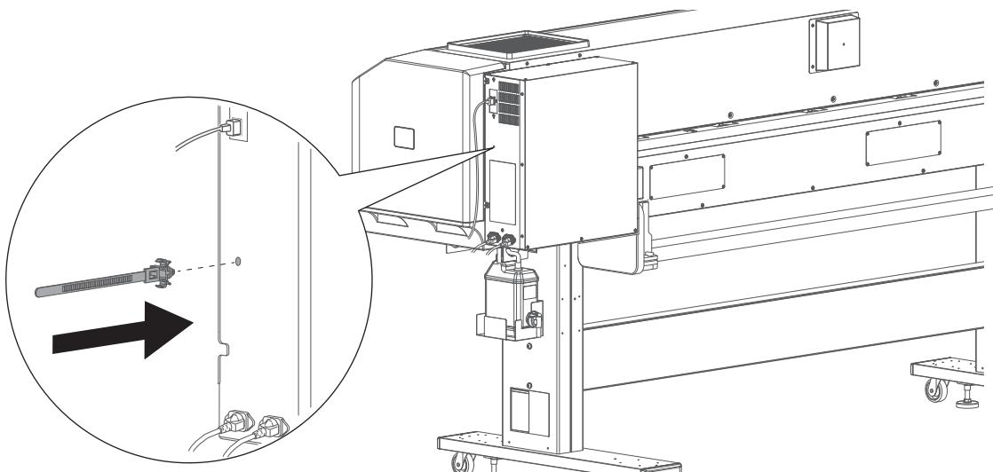
[3] Use the cable tie to secure the Ethernet cable to the printer.
