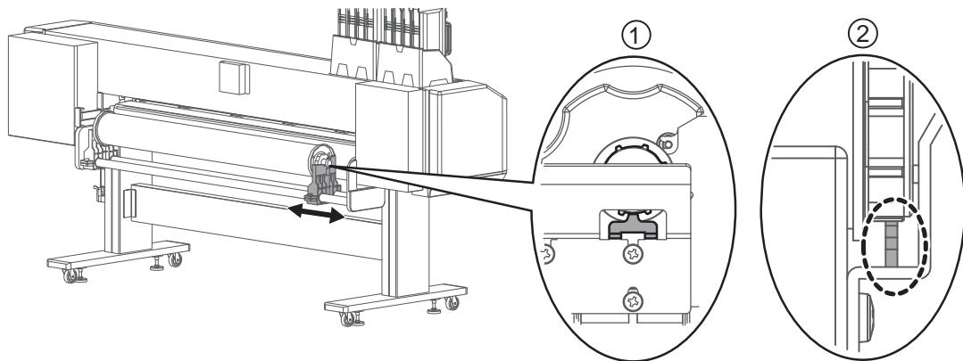
[4] Twist the knob bolt on the right side of the media holder clockwise to tighten.
