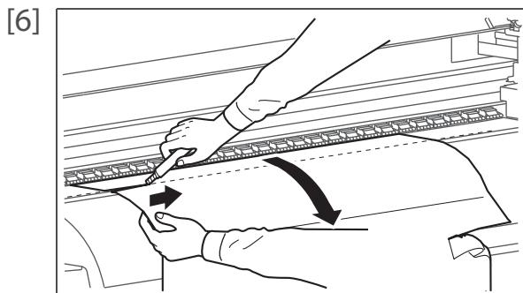
Pull the media towards you and use a cutter to cut the torn part of the media along the groove.
