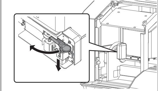
Press the cutter cap lightly, turn Cutter holder in the direction as illustrated below.
