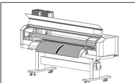
From the front side of the printer, pull the media for approximately 1 m.
