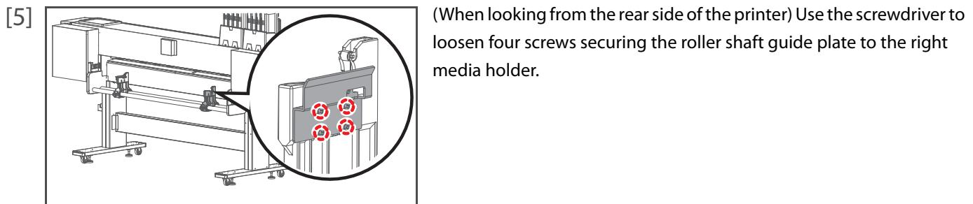
(When looking from the rear side of the printer) Use the screwdriver to loosen four screws securing the roller shaft guide plate to the right media holder.
