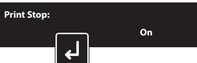
Sets whether or not to display "Roll Near End: \*m" (\* is replaced with a number between 1 and 10) before the length of the media that is counted inside the printer becomes 0.
