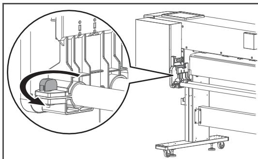
Twist the knob bolt on the left side of the media holder anticlockwise to loosen.
