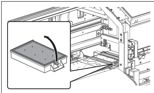
Pull the tab up of the absorption material for the flushing box, and release the hook.
