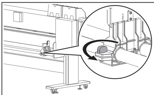
Twist the knob bolt on the right side of the media holder anticlockwise to loosen.
