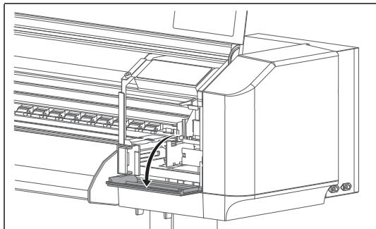
[3] Check the absorption material for the flushing box.
