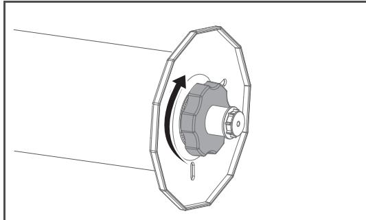
Twist the handle clockwise to lock the flange.
