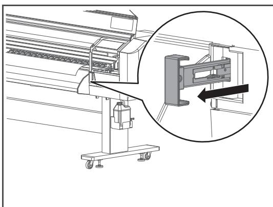
(To cancel the individual pressure rollers) From the front side of the printer, pull the media feed lever towards you as much as possible to release the pressure rollers.
