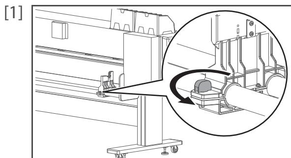
Twist the knob bolt on the right side of the media holder anticlockwise to loosen.
