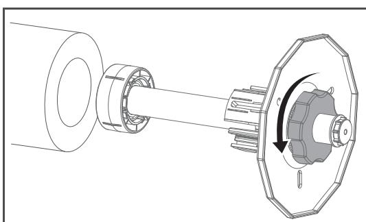
Push the media flange (×2) into the both ends of the media core.
