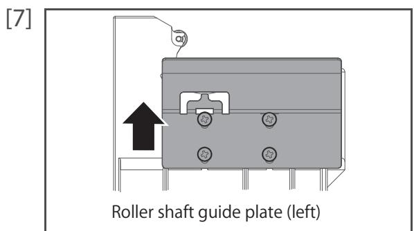
Do the same for the left media holder to slide up the roller shaft guide plate as far as it will go and tighten the screws.
