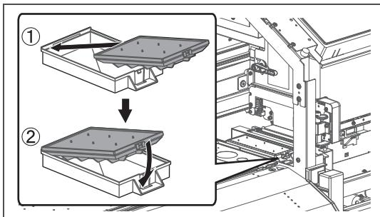
Attach new absorption material for the flushing box.
