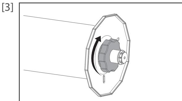
[3] Twist the handle clockwise to lock the flange.
