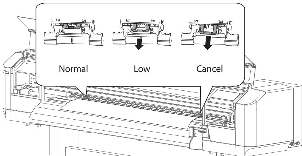
[4] (To cancel the individual pressure rollers) Push the media feed lever back to the original position to lock the pressure rollers.
