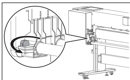
[2] Twist the knob bolt on the left side of the media holder anticlockwise to loosen.
