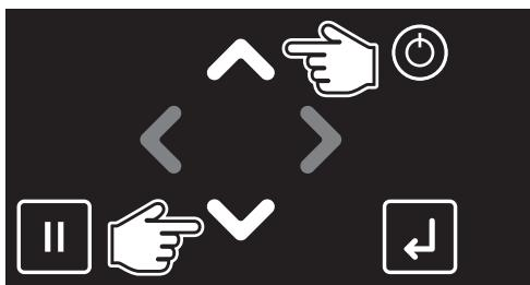
Long-touch or to feed a roll media until it reaches to the desired position.
