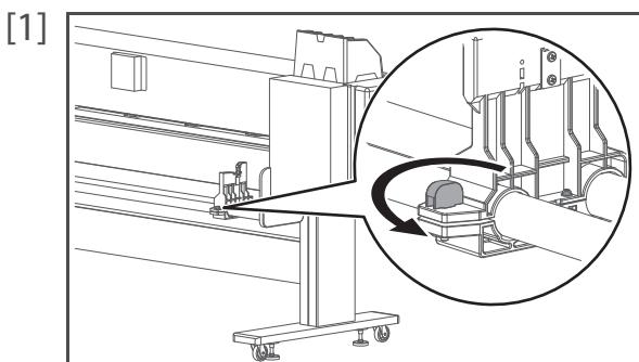
[1] Twist the knob bolt on the right side of the media holder anticlockwise to loosen.
