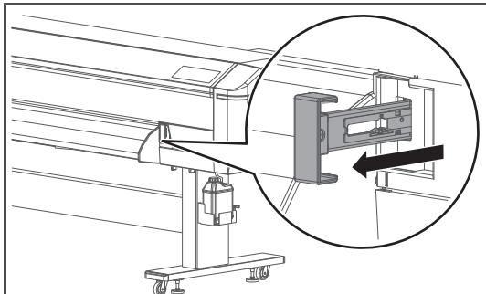
From the front side of the printer, pull the media feed lever towards you as much as possible to release the pressure rollers.
