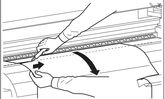
Pull the media towards you and use a cutter to cut the torn part of the media along the groove.
