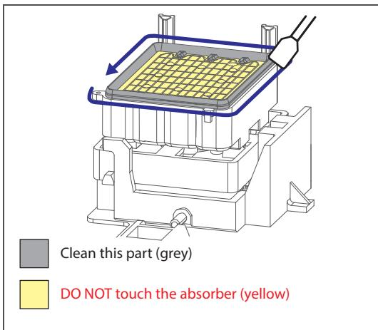
Use the cleaning stick to clean around the rubber part of the capping unit to remove the ink deposits and dust.
