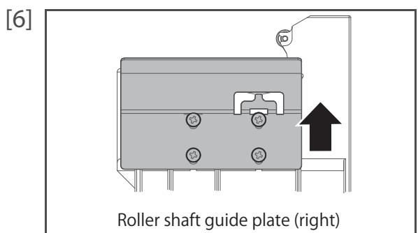
Slide up the roller shaft guide plate as far as it will go and tighten the screws.
