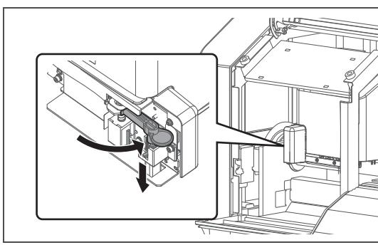
Press the cutter cap lightly, return Cutter holder to its initial position.
