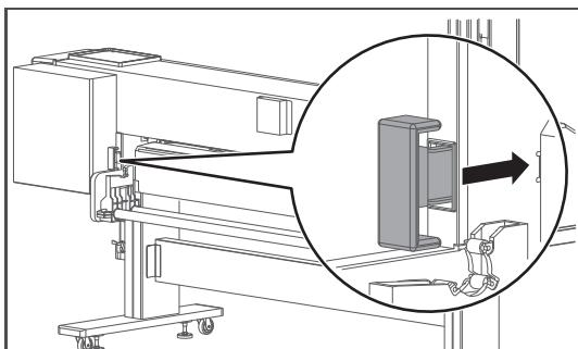
You can access to the media feed lever from the rear side of the printer.
