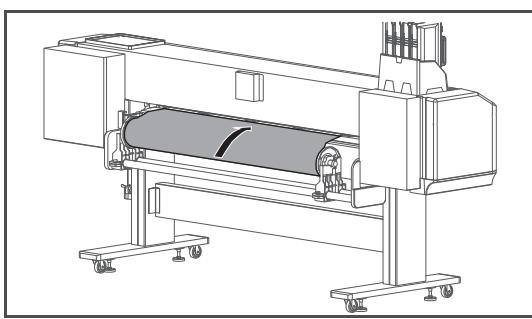
From the rear side of the printer, insert the front edge of the media into the media slot.
