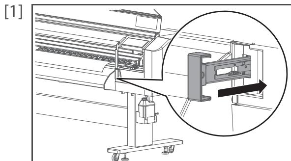
From the front side of the printer, push the media feed lever to hold the media flat with pressure rollers.
