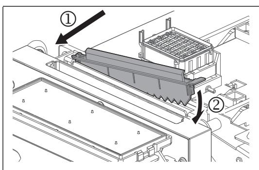
Attach an appropriate cleaning wiper to the wiper slot.
