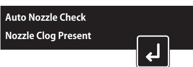
If the printer is unable to select a print head or a nozzle segment that works properly even after 3 cleanings, the message "Auto Nozzle Check Nozzle Clog Present" will appear on the operation panel.
