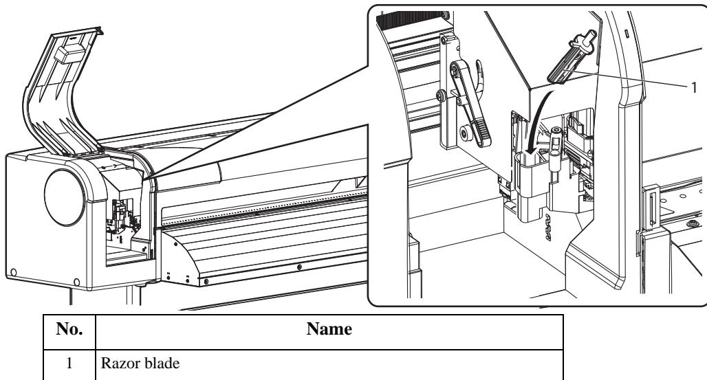
8. Press the tab of the cutter lightly, return the cutter holder to its initial position.
