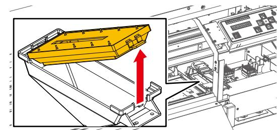
7 Install a new flushing box.
