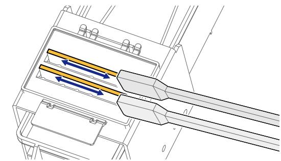
5 Use the cleaning stick to clean the parts around the capping unit to wipe off ink and dust.
