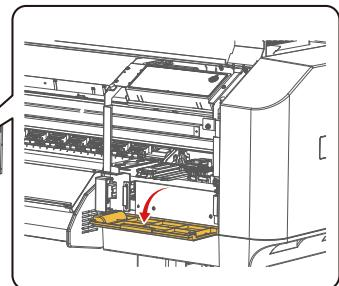
6 Pinch the wiper pad and lift it up to remove it.
