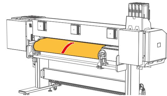
5 From the front side of the printer, pull the media for approximately 1 m.
