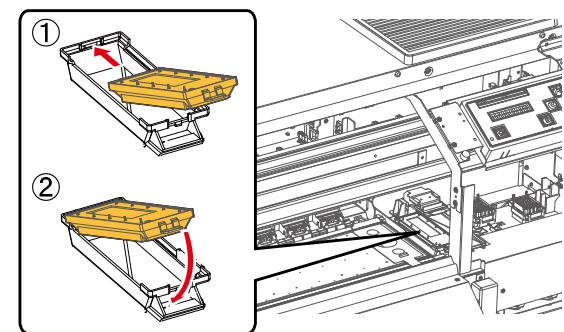
8 Fill 30 ml of maintenance cleaner into the flushing box.
