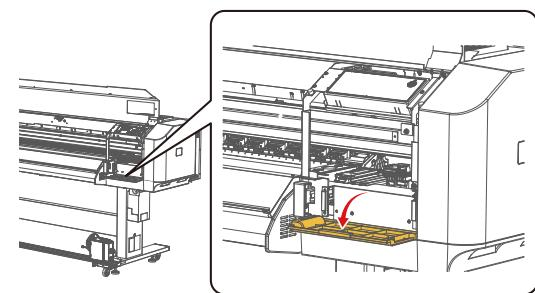
6 Fill about 20 ml of maintenance cleaner into the flushing box.
