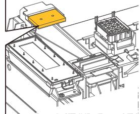
7 Insert the wiper pad into the pad slot from the top.
