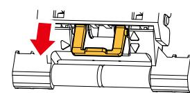
3. Push the media feed lever to lower the pressure rollers.
