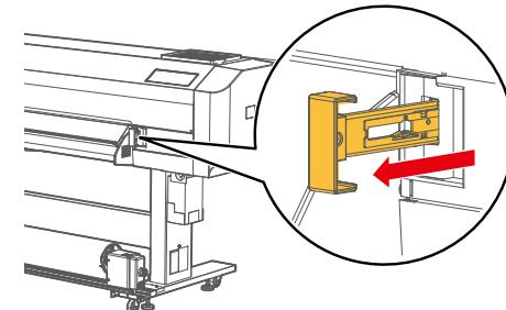
You can also access to the media feed lever from the rear side of the printer.
