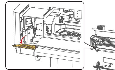
6 While holding the UV-LED unit, remove the filter.
