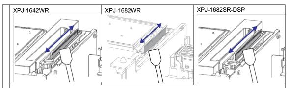
**Wipe the right side** of the wiper back and forth using a cleaning stick moistened with some cleaning fluid (DS3-CL1000E).
