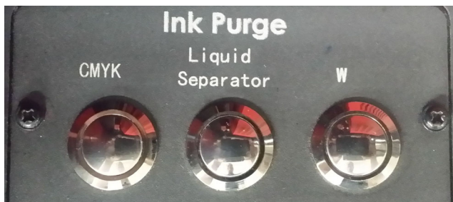
Figure 3-15: Liquid Separator - Empties Cyclonic Container
