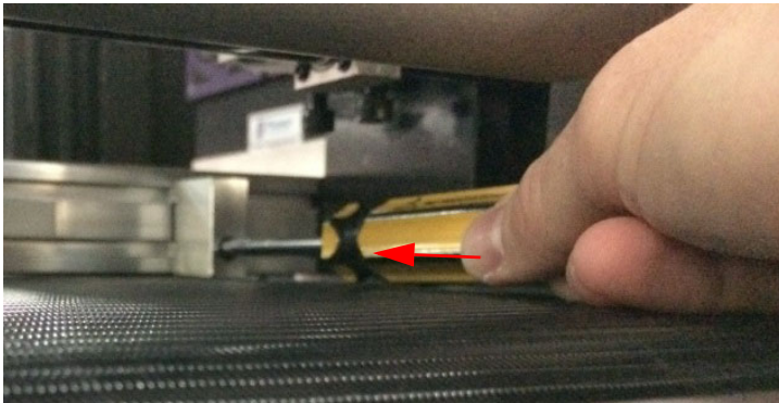
Figure 6-20: Loosen Screws on Guide Blocks
