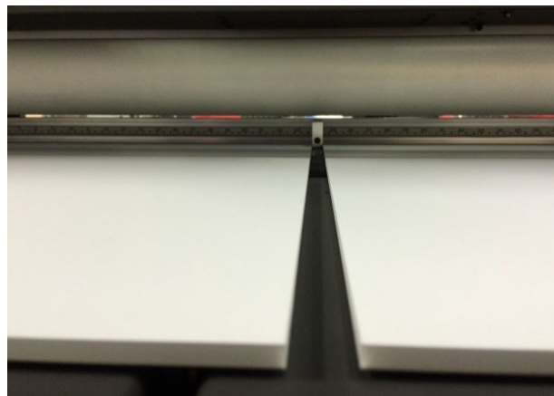
Figure 6-22: Press Each Board Against a Guide Block
