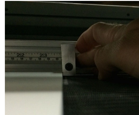
Figure 6-21: Place Guide Blocks Against Boards
