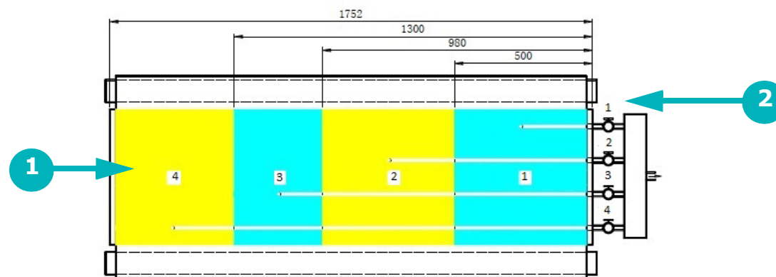
Figure 5-14: Vacuum Media Belt and Platen Vacuum Chamber Layout (Top View)
